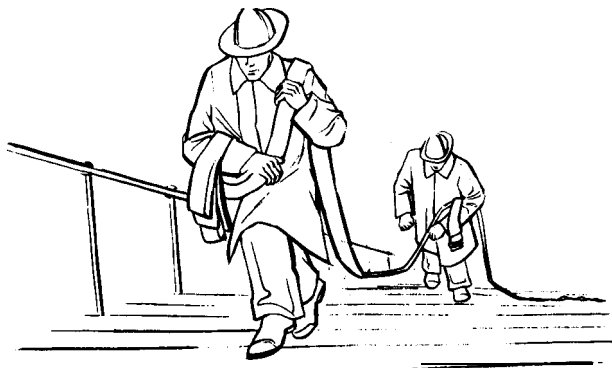
Figure 4-25. Advancing a hose up a stairway.
